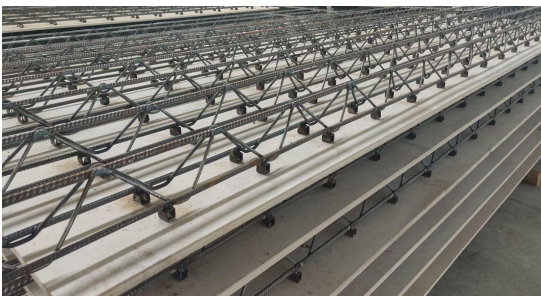
Reinforced truss floor decking
